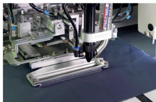
Pocket opening with laser
